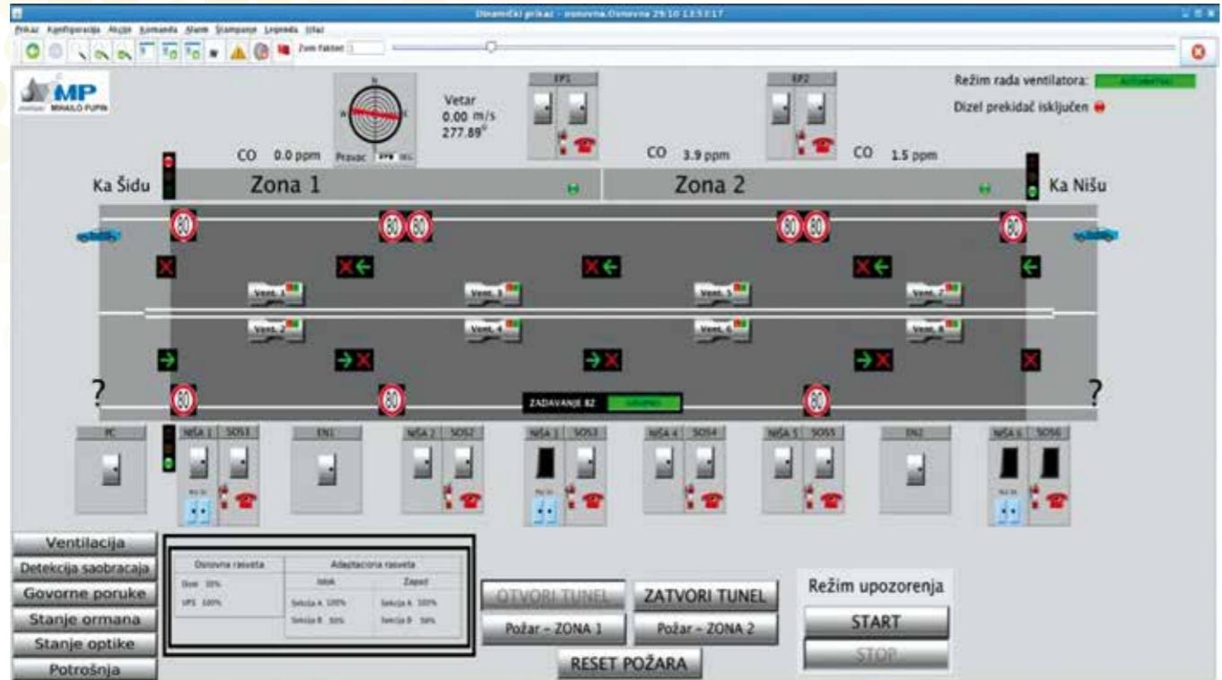
Comprehensive dedicated SCADA (Supervisory Control And Data Acquisition) solution for management of traffic tunnels provides real-time data presentation and easy execution of complex control functions using specialized dialogs.
