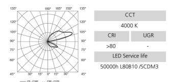
**GENERAL** Wall mounted luminaire for direct or indirect illumination, particularly appropriate for recovery hospital rooms.
