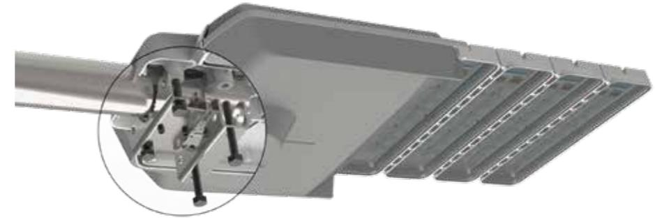
Mounting directly on arm  $\varnothing 60$  mm (side entry 42- 60 mm) with possibility to adjust the angle  $\pm 10^\circ$  in  $5^\circ$  increments.
