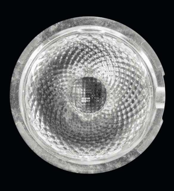
**LFO** Lens made of PMMA, retracted from the bottom surface of the luminaire, emitting light through perforation on the surface. Retraction from the perforation enables invisibility of the light source, providing full visual comfort. Light from nowhere.
