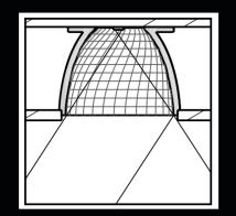
**MD** Micro downlighter reflectors with complex surfaces geometry of micro facets allow precise shaping of light beam. Angles of direct light beam and light reflected from reflector are almost perfectly aligned, providing sharp cut off for full visual comfort (UGR < 19).
