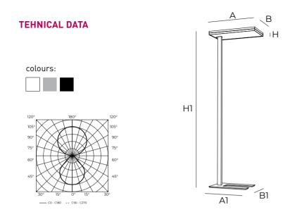
Dimensions A/A1/B/B1/H/H1 615 / 500 / 325 / 335 / 44 / 1950 mm Ingress protection rating Finish white, gray, black Weight 16kg Luminaire luminous flux (t<sub>a</sub>=25°)
