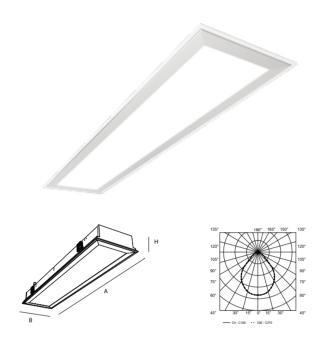
Dimensions A/B/H 1195x295x108mm Cut -out dimensions a/b/h 1180x280x160mm Ingress protection rating Impact resistance IK10 antibacterial white epoxy polyester powder Finish Weight Luminaire luminous flux (t = 25°) 7350/8700lm Total power 74/73W Luminaire efficiency 100/119 lm/W Light colour temperature 4000K CRI >90/ >80 UGR <19/<22 LED service life 60.000h(L80B10) SDCM 3 220-240V, 50-60Hz Power supply ECG, DALI Control gear
