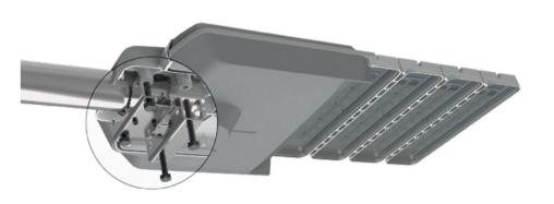
Mounting directly on arm Ø60 mm (side entry 42- 60 mm) with possibility to adjust the angle ±10° in 5° increments.
