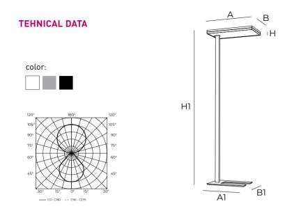
Dimensions A/A1/B/B1/H/H1 Ingress protection rating 615 / 500 / 325 / 335 / 44 / 1950 mm Finish white, gray, black Weight 16kg Luminaire luminous flux (t<sub>a</sub>=25°) Total power 11295 lm 95W Luminaire light output Light colour temperature /CRI LED service life 119lm/W 4000K / >80 50000 L70B10/3SCDM Power supply 220-240 V 50-60 Hz Control gear DALI Touch Dimm
